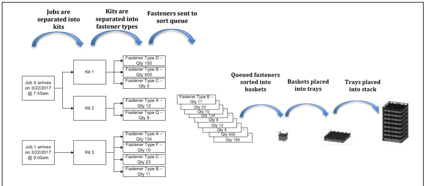
The full stacks then flow to the acetone cleaners, adhesion promoters, and bagging stations (per Steps 3-5 in Figure 1). Once stacks reach the bagging station (Step 6), trays are removed from stacks, baskets are removed from trays, fasteners are emptied from baskets and bagged, and bags of fasteners are grouped into their respective kits and delivered to the production line for installation on the aircraft.
