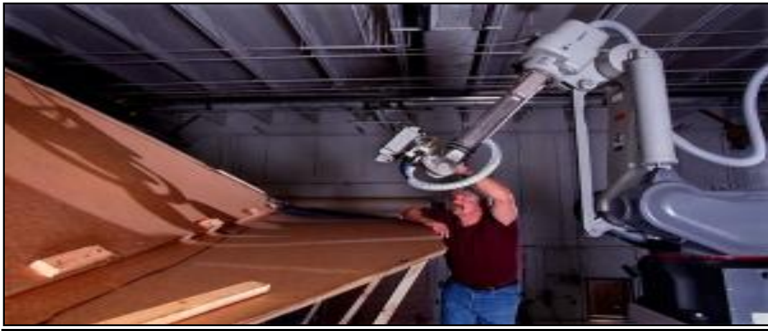
Figure 24. Explosion Proof Robot.
